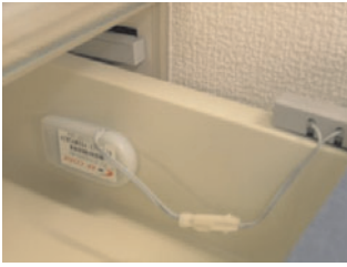
Fig. 5. Magnet sensor on a drawer.
