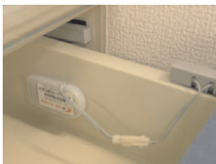
Fig. 5. Magnet sensor on a drawer.
