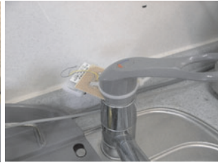
Fig. 6. Limit switch sensor on a faucet.
