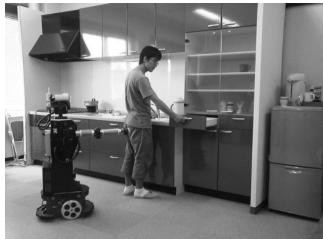
Fig. 9. Cooking-support robot recommending a presumed next action by voice and gesture.
